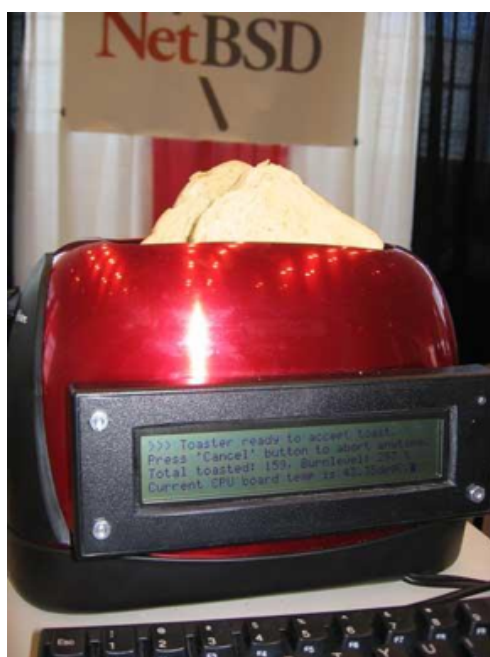
Figure 3. NetBSD Toaster with the TS-7200 ARM9 SBC
