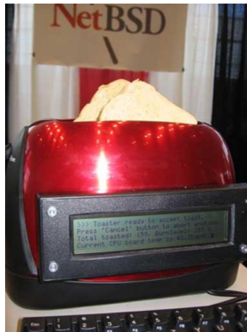
Figure 3. NetBSD Toaster with the TS-7200 ARM9 SBC
