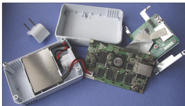
Figure 2. The SheevaPlug Disassembled. The circuit board on the far right contains the development hardware (serial console, JTAG interface, USB, and SDIO interfaces). The circuit board in the center holds the Marvell processor, Ethernet port, USB port, and system memory. The power supply is under the metal plate in the case on the left side
