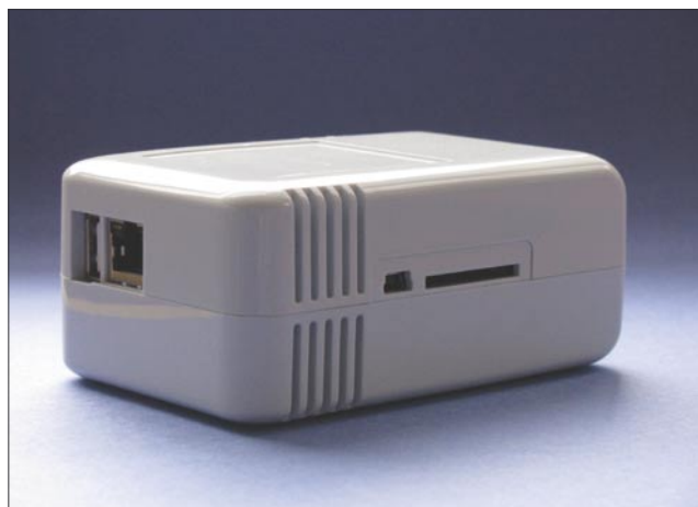
Figure 1. The SheevaPlug Computer. The USB and GigE ports are on the left, and the debug devices (mini-USB and SDIO memory card) are on the right
